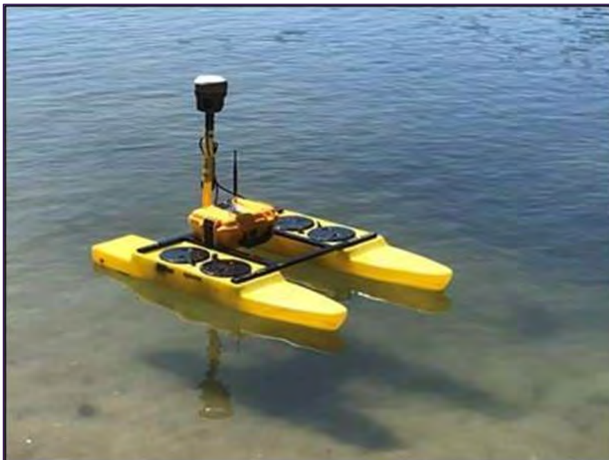
Figure 3.23 Photograph of the Hydrone USV used at Hemerdon MWF for bathymetric surveying (Mining Plus, 2021b)
