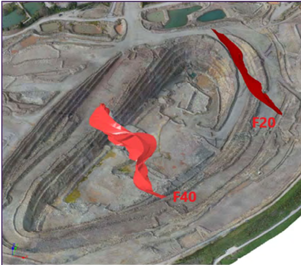
Figure 3.21 Plan view of current open-pit showing Faults F20 and F40
